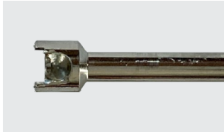
Ball Driver Deformed due to misuse
