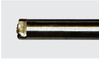
Instrument shaft Fractured due to over torque
