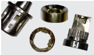
Manual Handle Broken, decreased retention
