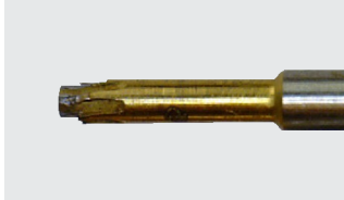
Screwdriver Twisted tip due to overload
