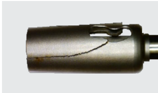
Drill Extender Corrosion, fracture
