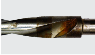
Twist Drill – Multiple Use Corrosion
