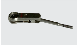
Ratchet Broken pin due to lack of lubrication
