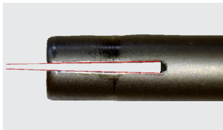
Tack positioning instrument Corrosion, deformed
