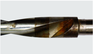
Twist Drill – Multiple Use Corrosion
