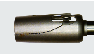
Drill Extender Corrosion, fracture
